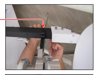
Step 18 Gently, hand rotate the RF FEED to make sure it rotates freely.
