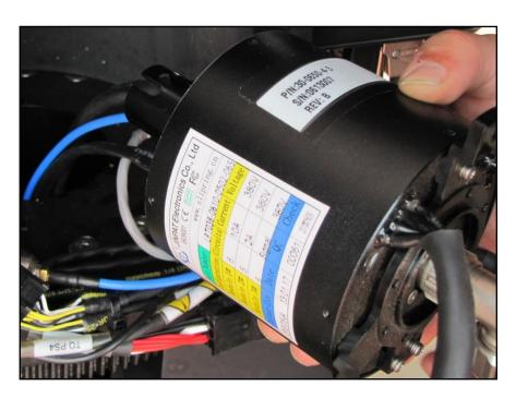
Figure 1-1: Slip Ring/Rotary Joint Assembly
